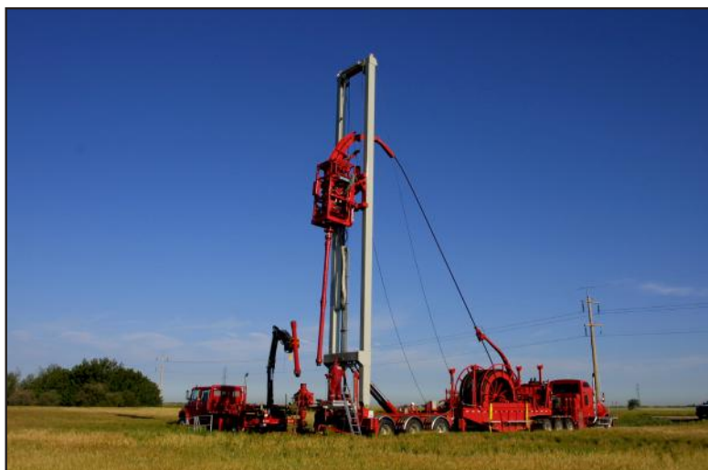
Figure a-44: a MaST TyPe Coiled Tubing unit
