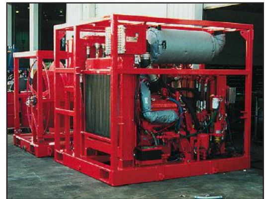
Figure a-5: Coiled Tubing unit Prime Mover
