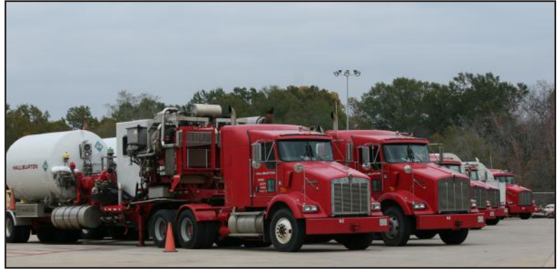
Figure a-48: a niTrogen uniT
