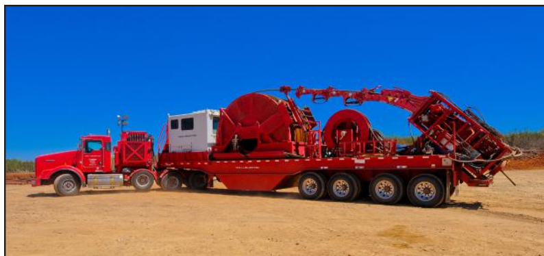
Figure a-2: Truck Mounted Coiled Tubing Unit
