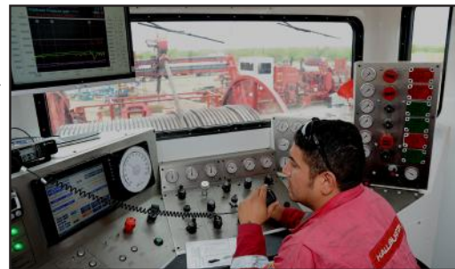
Figure a-13: Inside a Coiled Tubing unit
