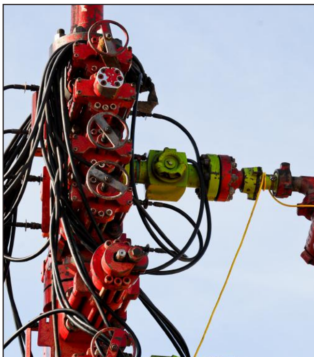
Figure a-28: loWer kill line uSed For reTurnS
