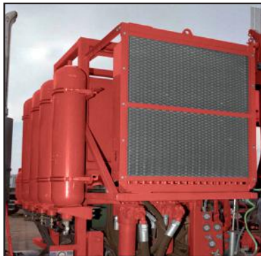
Figure a-31: aCCuMula Tor SySTeM, TruCk MounTed
