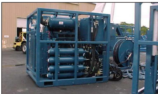
Figure a-30: aCCuMula Tor SySTeM
